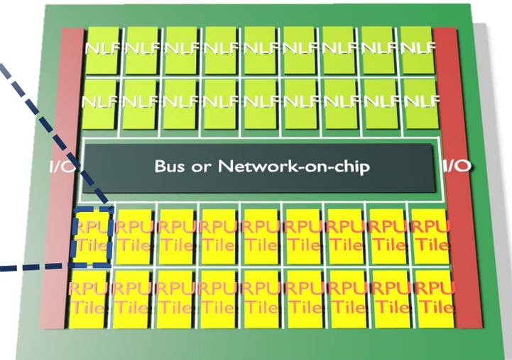
\*RPU = Resistive processing unit, NLF = Non-linear function, NoC = Network-on-chip
