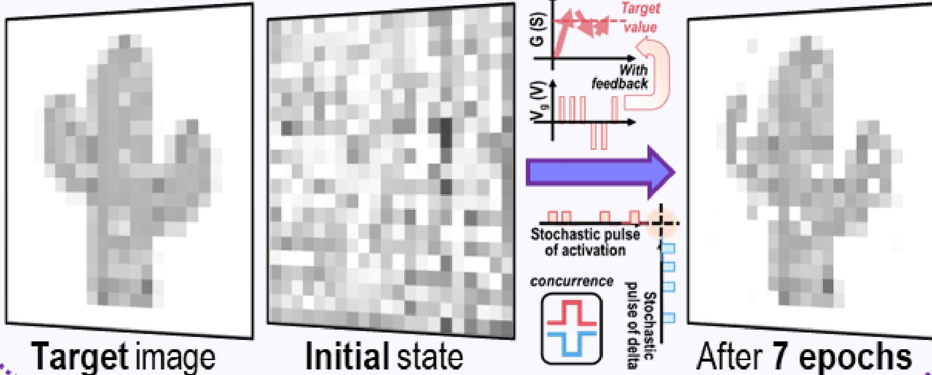
The largest-scale hardware demonstration of *in-situ* learning, involving 441 selector-free devices, which is a state-of-the-art result
